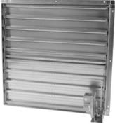
This damper has a flanged frame and is designed to fit the inside flanges of the optional wall housing or wall mounting collar. The frame and blades are constructed of galvanized steel and are rated to 3000 FPM with proper clearance as provided by all factory accessories. The damper body recesses into the opening for a flush appearance.
