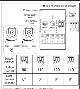
Factory setting: 110CFM ( with 6" duct)
