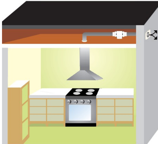
Domestic - Range Hood Exhaust
