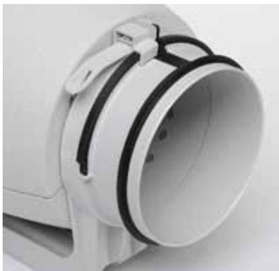
Bi-material inlet and outlet incorporating a flexible washer to facilitate installation, absorb vibrations and provide a virtually **air-tight** seal.
