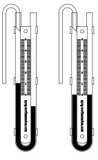
Working: Fan is operating when liquid levels are uneven. Not Working: Fan may not be operating correctly if liquid
