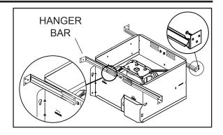
2b. Extend the hanger bars to the width of the framing. Position the ventilator with the hanger bar tabs wrapped around the bottom edge of the framing, holding the ventilator in place.
