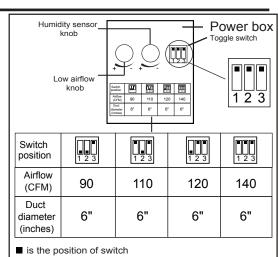
Factory setting: 110CFM (with 6" duct ) HVI Certified performance based on HVI Procedures 915, 916, and 920.
